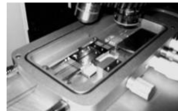
Fig. 9. Photograph of the sample chamber of the Linkam CAP 500 heating-cooling stage.
