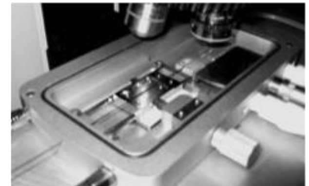
Fig. 3. Photograph of the sample chamber of the heating-cooling stage.
