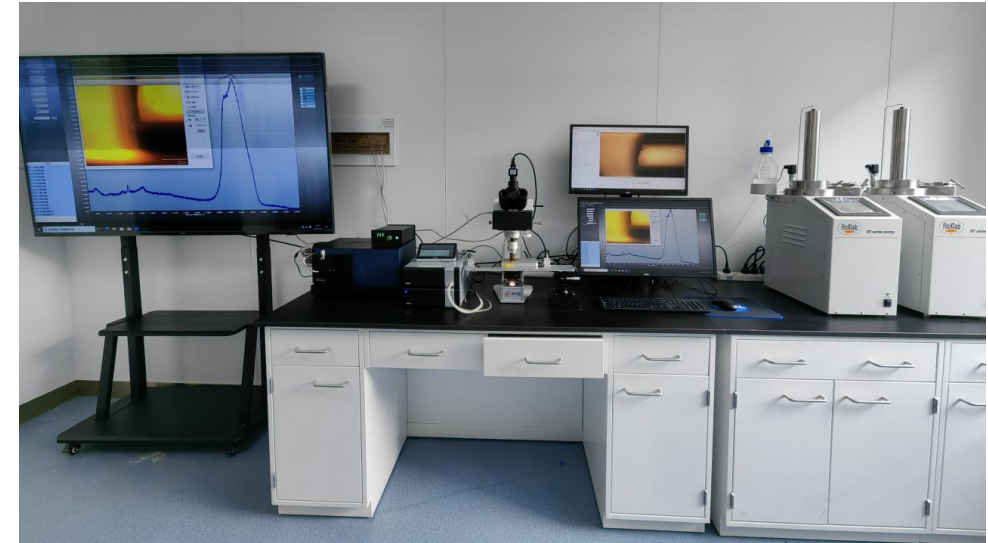
Full Visual Microtubule Raman Microprobe Under HT-HP Control
